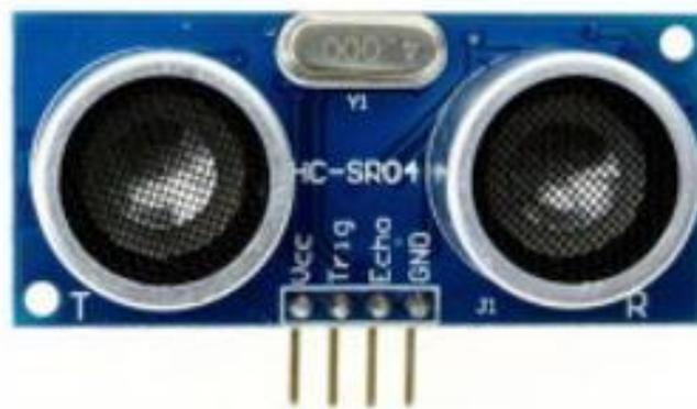
**Gambar 2. Sensor ultrasonik**
