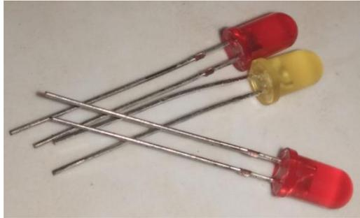
Gambar 10. LED (*Light Emitting Diode*)
