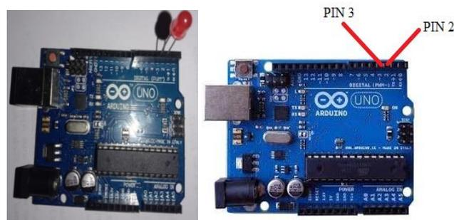
Gambar 39. pin Indikator LED
